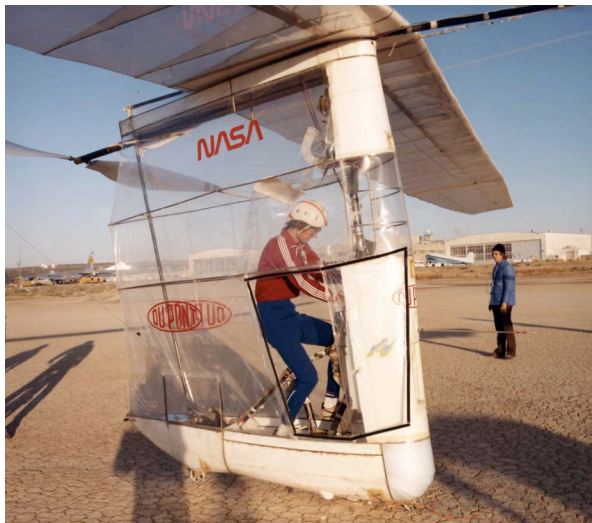
Bryan Allen, about to pedal the Gossamer Albatross, with its 96 foot wingspan. It weighed only 66 pounds. Allen was both the pilot and the engine. (NASA photo by Jim Moran)
