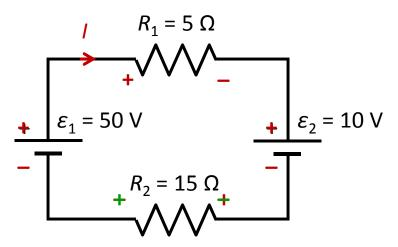
Calculate the current *I* in the circuit
