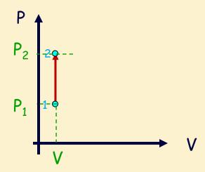
Comparing it to last slide where we had a constant pressure process (and same  $T_1$  &  $T_2$ ): Less heat is required to raise T at const. volume than at const. pressure
