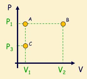
→ to change the system from C to B, energy must be added to system
