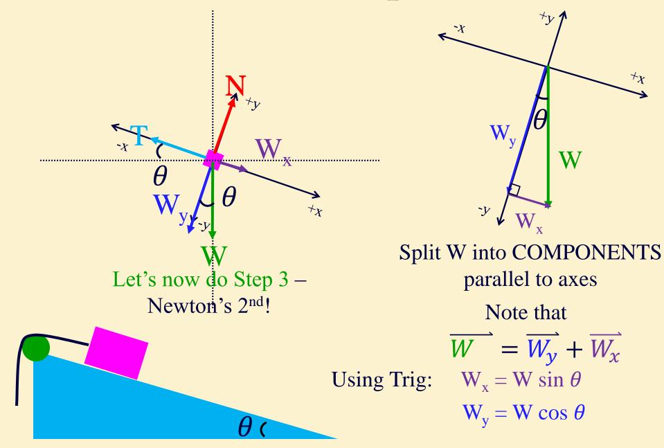
Calculate tension necessary to keep the 5 kg block from sliding down a frictionless incline of 20 degrees.
