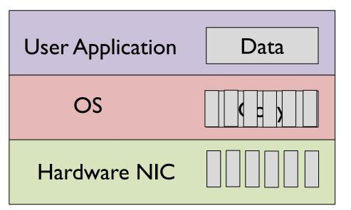
Packet processing in OS incurs high latency, cannot support high throughput, and leads to high CPU utilization.
