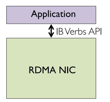
Applications bypass the kernel and interact directly with the RDMA NIC using the **IB verbs** API provided by the NIC driver.
