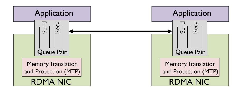
Connection establishment requires out-of-band exchange of node identifiers, QP id, and remote keys.
