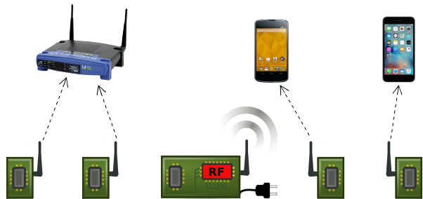
Figure 1: Passive Wi-Fi architecture. The passive Wi-Fi devices perform digital baseband operations like coding, while the power-consuming RF functions are delegated to a plugged-in device in the network.
