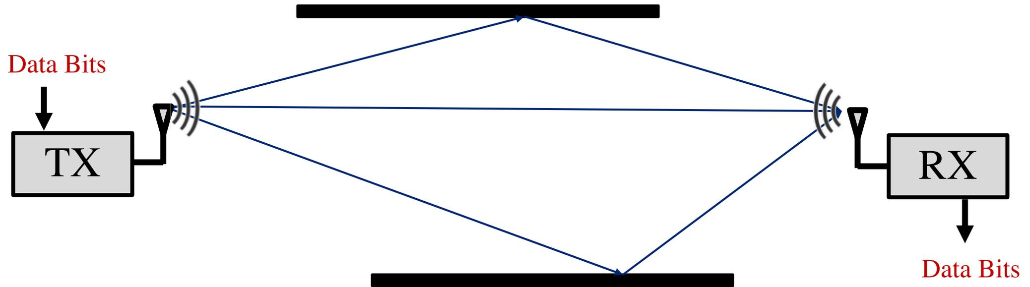
**Multipath Propagation:** radio signal reflects off objects ground, arriving at destination at slightly different times
