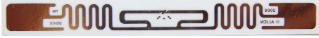
Figure 9—Commercial UHF RFID Used in Experiments: Alien Squiggle General Purpose UHF RFID
