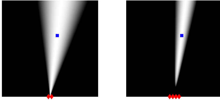
Figure 6: Larger antenna array demonstrating higher resolution; \frac{\lambda}{2} -spaced antenna arrays with 2 and 4 antennas, respectively
