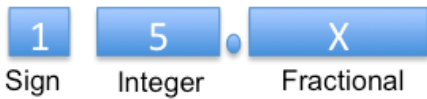
Fig. 13. Fixed point representation with variable number of bits to represent the fractional part.
