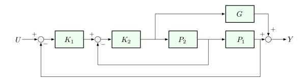
Compute the transfer function from the input U to the output Y.
