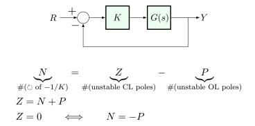
Nyquist Stability Criterion. Under the assumptions of the Nyquist theorem, the closed-loop system (at a given gain K) is stable *if and only if* the Nyquist plot of G(s) encircles the point -1/K P times *counterclockwise*, where P is the number of unstable (RHP) open-loop poles of G(s).
