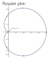
$#(\circlearrowright \text{ of } -1/K) = #(\text{RHP CL poles}) - \underbrace{\#(\text{RHP OL poles})}_{=0}$
