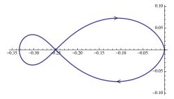
$$\begin{array}{l} \#(\circlearrowright \text{ of } -1/K) \\ = \#(\text{RHP CL poles}) \\ - \underbrace{\#(\text{RHP OL poles})}_{=1} \end{array}$$
