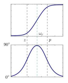
For best effect on PM,  $\omega_c$ should be halfway between zand p (on log scale):
