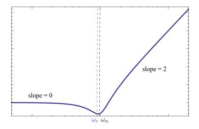
For a stable real zero, the magnitude slope "steps up by 2" at the break-point.
