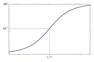
For a stable real zero, the phase "steps up by  $90^{\circ}$ " as we go past the break-point.
