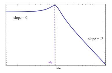
For a stable real pole, the magnitude slope "steps down by 2" at the break-point.
