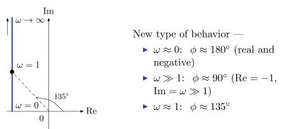
For a RHP zero, the phase starts out at  $180^{\circ}$  and goes down by  $90^{\circ}$  through the break-point ( $135^{\circ}$  at break-point).
