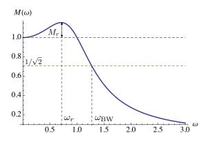
$\omega_r$  – resonant frequency  $M_r$  – resonant peak  $\omega_{\rm BW}$  – bandwidth
