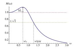
small  $M_r \longleftrightarrow$  better damping large  $\omega_{\rm BW} \longleftrightarrow$  large  $\omega_n \longleftrightarrow$  smaller  $t_r$
