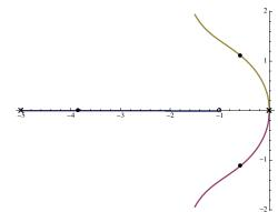
— for this value of p, the root locus is different, not nearly as nicely damped as for p = 10.
