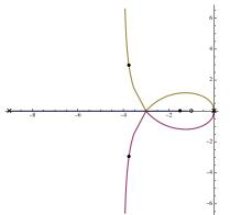
— for this value of p, the branches meet (*break in*) and separate (*break away*) at the same point on the real axis.
