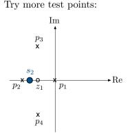
$\angle (s_2 - z_1) = 180^{\circ} \quad (s_2 < z_2)$  $\angle (s_2 - p_1) = 180^{\circ} \quad (s_2 < p_1)$  $\angle (s_2 - p_2) = 0^{\circ} \quad (s_2 > p_2)$  $\angle (s_2 - p_3) = -\angle (s_1 - p_4)$ (conjugate poles cancel)
