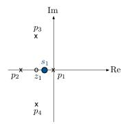
$$\angle (s_1 - z_1) = 0^{\circ} \quad (s_1 > z_1) \angle (s_1 - p_1) = 180^{\circ} \quad (s_1 < p_1) \angle (s_1 - p_2) = 0^{\circ} \quad (s_1 > p_2) \angle (s_1 - p_3) = -\angle (s_1 - p_4) (\text{conjugate poles cancel})$$
