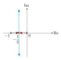
(s = -1/2 is the point of breakaway from the real axis)
