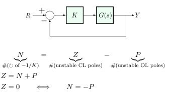
Nyquist Stability Criterion. Under the assumptions of the Nyquist theorem, the closed-loop system (at a given gain K) is stable if and only if the Nyquist plot of G(s) encircles the point -1/K P times counterclockwise, where P is the number of unstable (RHP) open-loop poles of G(s).
