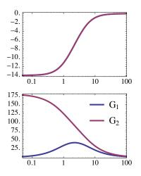
Among all transfer functions with the same magnitude plot, the one with only LHP zeros has the minimal net phase change as  $\omega$  goes from 0 to  $\infty$  — hence the term minimum-phase for LHP zeros.
