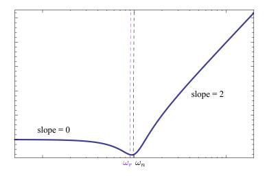
For a stable real zero, the magnitude slope "steps up by 2" at the break-point.
