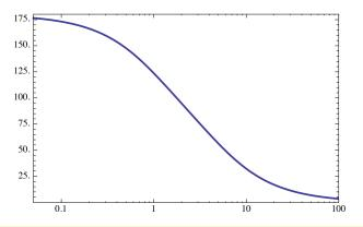
For a RHP zero, the phase plot is similar to what we had for a LHP pole: goes down by  $90^\circ$  ... However, it starts at  $180^\circ$ , and not at  $0^\circ$ .
