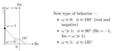
For a RHP zero, the phase starts out at  $180^{\circ}$  and goes down by  $90^{\circ}$  through the break-point ( $135^{\circ}$  at break-point).
