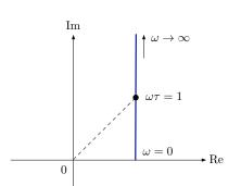
► For small  $\omega$  (below break-point),  $\phi \approx 0^{\circ}$
