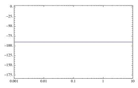
Phase:  $\angle K_0(j\omega)^n = \angle (j\omega)^n = n\angle j\omega = n \cdot 90^\circ$ — this is a constant, independent of  $\omega$ .
