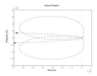
We have P = 2 (from the compensator), and we do see that N = -2, given Z = 0. The system is stable, but there is virtually no gain or phase margin.
