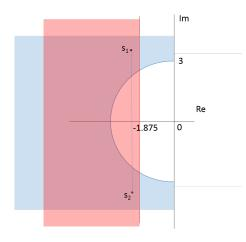
The poles of H(s) are the roots of  $s^2 + 4s + 16$ , which can be computed to be  $s_{1,2} = -2 \pm 2\sqrt{3}$ . they are plotted in the complex plane and found to be in both of shaded regions. Hence the given system satisfy these specs.
