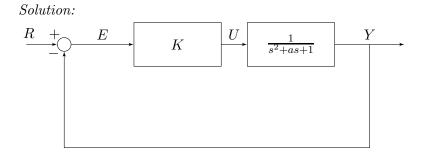
b) Derive the transfer function of the closed-loop system from r to y.
