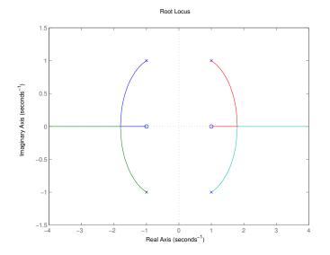
b) open-loop poles:  $1 \pm j$  from the attached SRL, we see that for every  $\rho$ , we assign the LHP pole for the CL system (due to symmetry vs imaginary axis)
