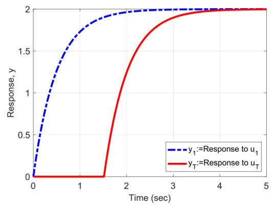
$\dot{y}(t) + 2y(t) = 4u(t)$ with y(0) = 0. Inputs are  $u_1(t) = 1$ and  $u_T(t) := u_1(t - T)$ . Time shift is T = 1.5 sec.
