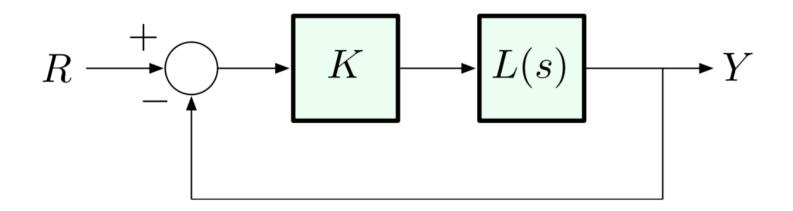
(a) If L has 5 LHP poles, 2 RHP poles, and 7 LHP zeros, is the closed-loop system stable for very large K>0?(b) If L has 4 LHP poles, and 2 LHP zeros, is the closed-loop system stable for very large K>0?
