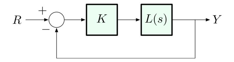
(a) Solve the closed-loop poles as a function of K.(b) Draw the root locus.
