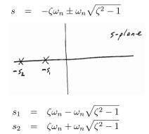
In both the overdamped and critically damped cases the step response does not oscillate
