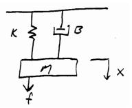
Suppose M, K are given. How should you choose B (shock absorber) so that the P.O. to a unit step is less than  $\sim 4\%$ . Example:
