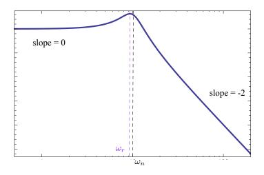
For a stable complex pole, the magnitude slope "steps down by 2" at the break-point.
