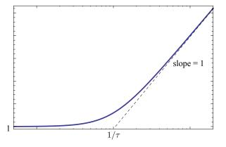
For a stable real zero, the magnitude slope "steps up by 1" at the break-point.
