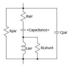
Capacitor Instance Parameters
