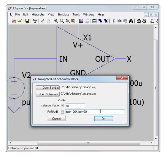
Note that is dialog also allows you to enter parameters to pass to this instance of the circuitry in preamp.asc.
