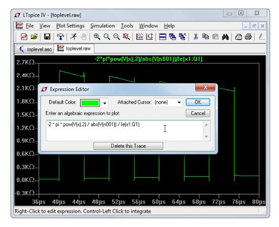
The difference of two voltages; e.g., V(a)-V(b); can equivalently written as V(a,b). The following functions are available for real data:
