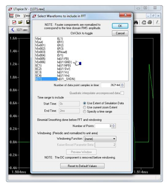
LTspice uses a proprietary FFT algorythm that allows an arbitrary number of datapoints, i.e., not limited to a power of 2.
