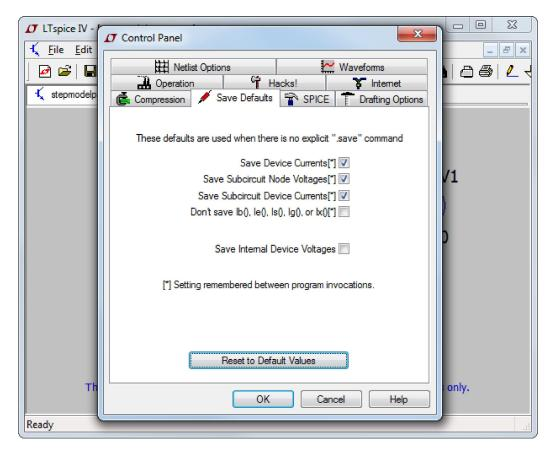
Save Device Currents: Check this so that you can plot device and terminal currents. You will also need it to be able to plot dissipation.
