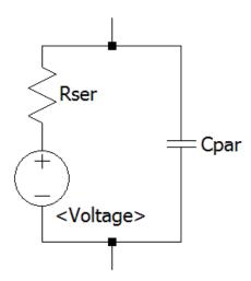
Voltage sources have historically been used as the current meters in SPICE and are used as current sensors for current-controlled elements. If Rser is specified, the voltage source can not be used as a sense element for F, H, or W elements. However, the current of any circuit element, including the voltage source, can be plotted.
