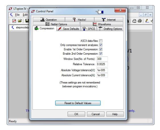
LTspice compresses the raw data files as they are generated. A compressed file can be 50 times smaller than the un-compressed one. This is a lossy compression. This pane of the control panel allows you to control how lossy the compression runs.
