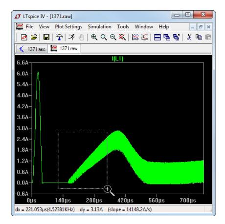
Note that the size of the zoom box is displayed on the status bar at the bottom so that you can quickly measure differences without setting up attached cursors.
