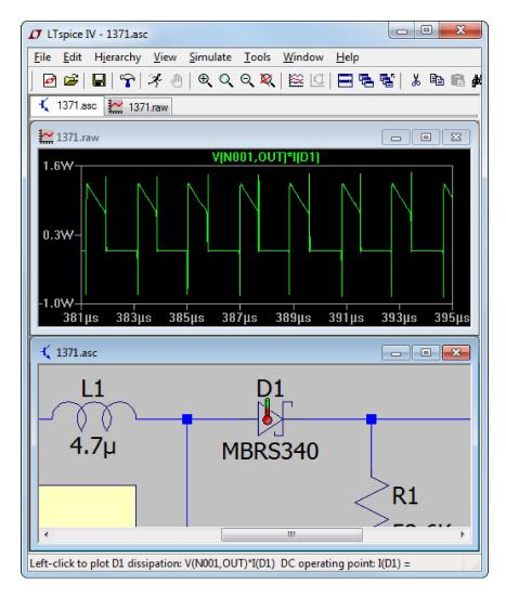
You can also probe the current in a wire. To do this, hold down the Alt key and click on the wire. The mouse cursor turns into a clamp on ammeter to indicate it's pointing at this current and the red arrow shows the direction of positve current.
