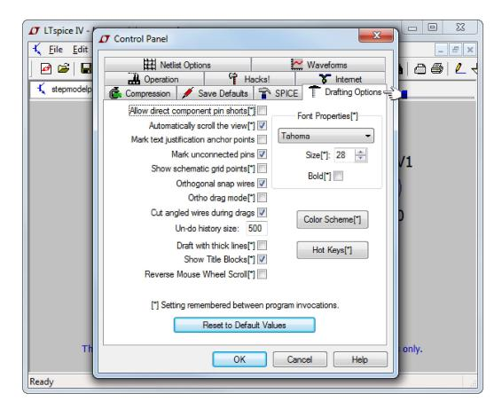
Allow direct component pin shorts: Normally you can draw a wire directly through a component and the wire segment shorting pins is deleted. If you check it, the shorting wire will not be automatically deleted.
