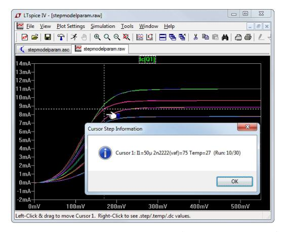
The attached cursors can also be used to readout which trace belongs to which run of a .step/.dc/.temp set of simulation runs. You can navigate the cursor from dataset to dataset with the up/down keyboard cursor keys and then right-click on the cursor to see the step information for that run.
