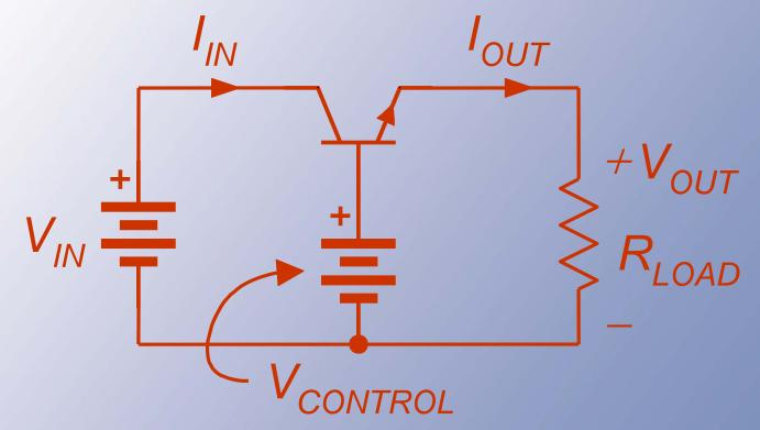
The emitter voltage follows the (low-power) base voltage.
