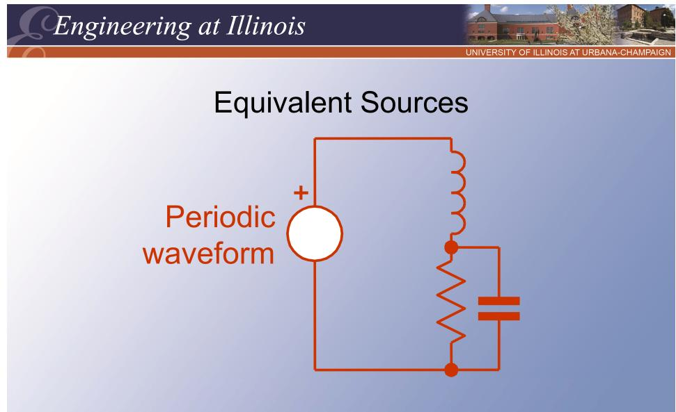
We can represent the periodic waveform with a Fourier series.
