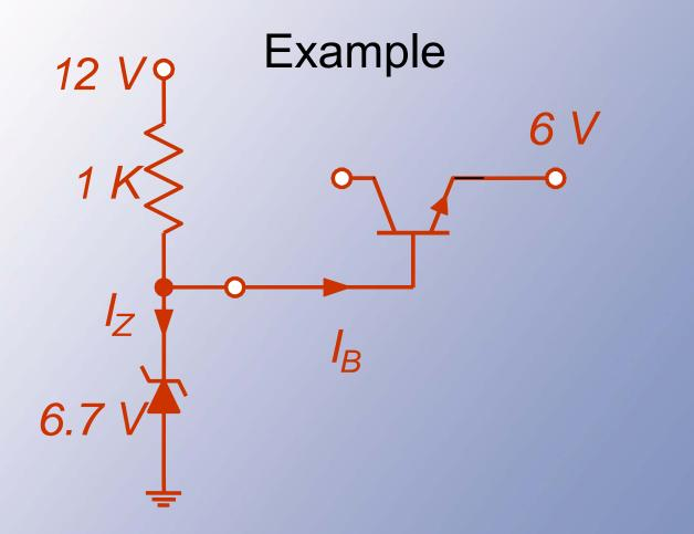
Here, a shunt regulator provides the reference voltage for a series regulator.
