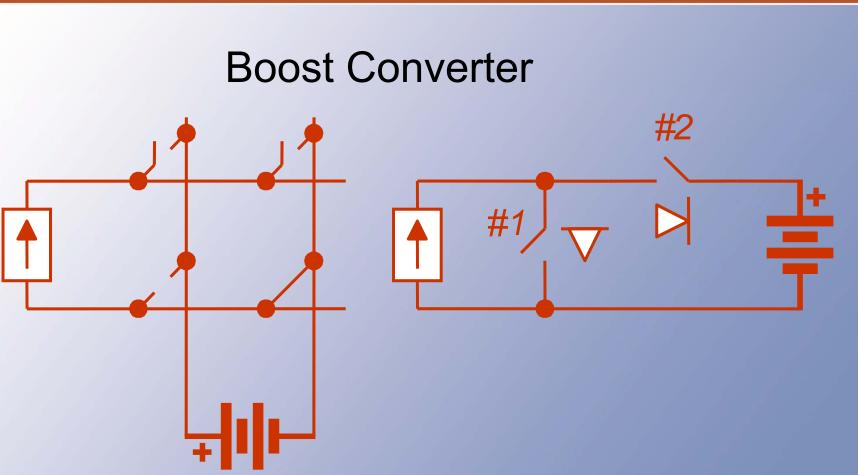
A boost converter is a buck converter flipped horizontally.
