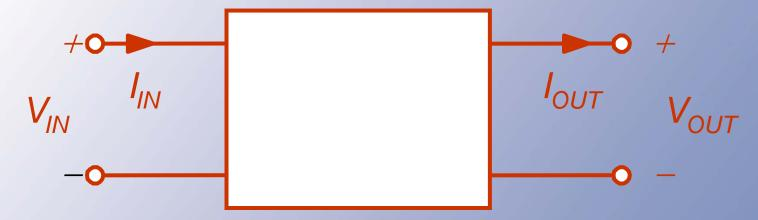
$$\begin{aligned} P_{in} &= V_{in} I_{in} = P_{out} = V_{out} I_{out} \\ \frac{V_{out}}{V_{in}} &= a & \frac{I_{in}}{I_{out}} = a \end{aligned}$$
