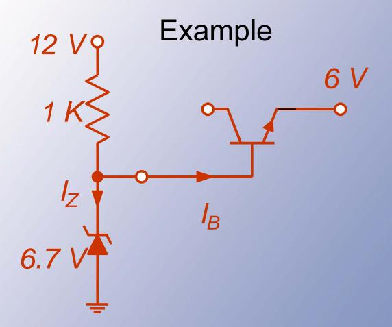
Here, a shunt regulator provides the reference voltage for a series regulator.
