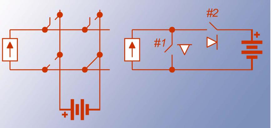
A boost converter is a buck converter flipped horizontally.
