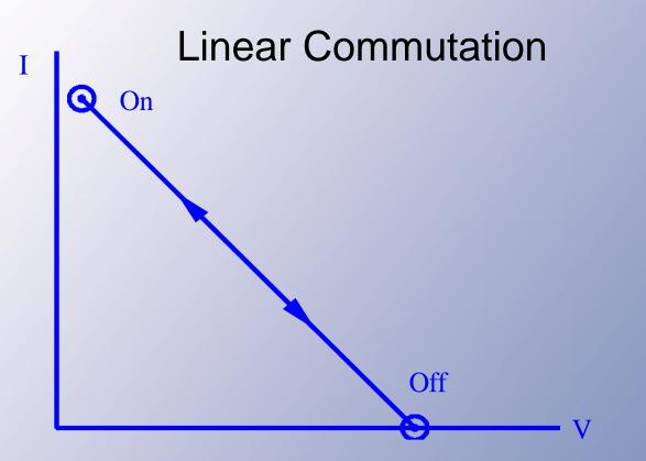
• The switching trajectory can be plotted: a straight line between on and off points.
