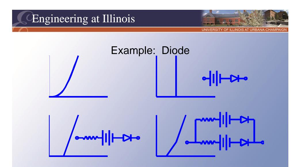
• Most static models are *piecewise* circuits, like these three.
