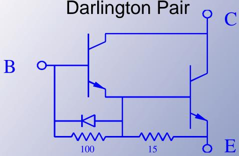
Manufacturers often add internal diodes and other parts to try to speed the action of a Darlington pair.
