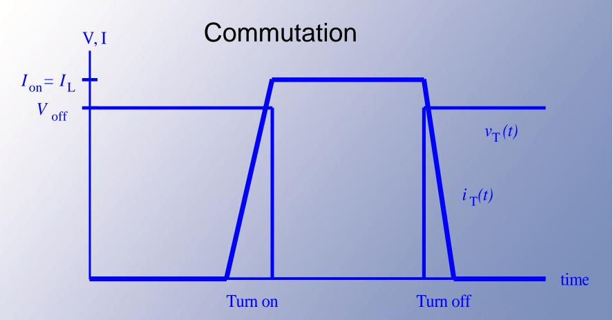
• Waveforms in a typical dc-dc converter show high voltages while the current changes.
