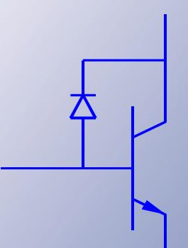
• Sometimes a diode is added to divert excess base current. (A "Baker clamp.")
