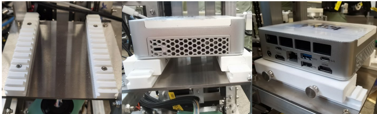
Figure 2.2.3.6 The picatinny rails(left), the mini-PC with sliders(middle) and the hand screw(right).
