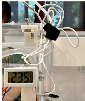
Figure 42: Temperature sensor works for open-loop feedback.
