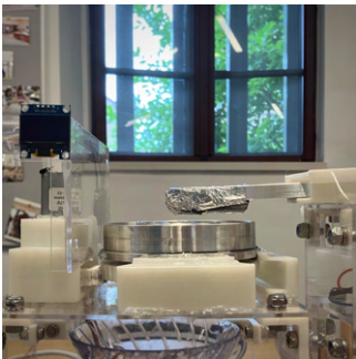
Figure 19: The hot water slider is wrapped with foil to prevent water overflow
