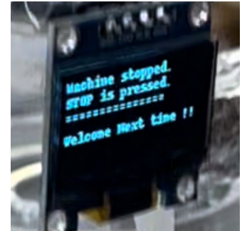
Figure 31: The machine stopped due to the emergency stop button is pressed.
