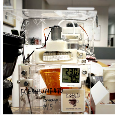
Figure 14: Gear Module Running In Practice, the 9kg torque force can deform the holder.
