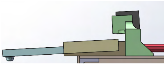
Figure 16: 3 degree inclination to self-clean left water
