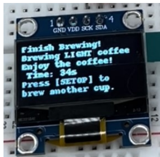
Figure 30: The coffee machine finishes brewing a cup of light-roasted coffee, using 34 seconds.
