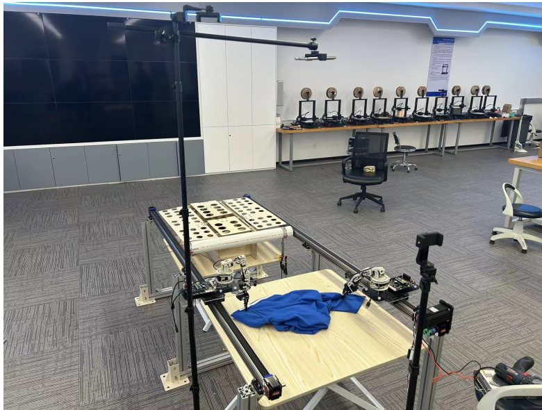
Figure 1.9 Vision System: Hanging Camera
