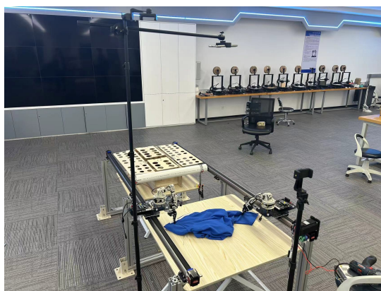
Figure 3.28 Structures of hanging camera(Two black camera stands)
