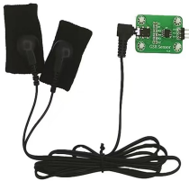
Figure 5: Skin Conductance Sensor
