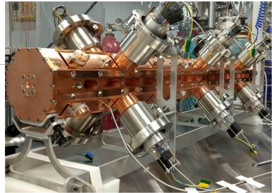
Starfire's prototype, compact 4 MeV D+ RFQ cavity
