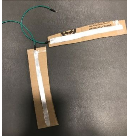
Design 2: X-Y Strip Sensor
