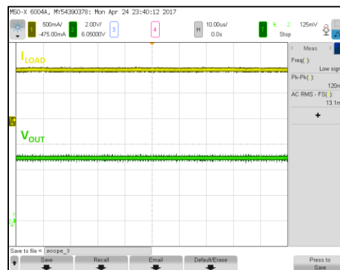
Figure 23: Output Voltage and Current Waveform (12 V AC-DC converter)
