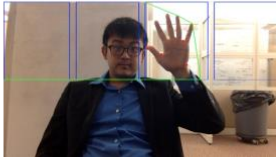
Figure 14. Contour Detection with Localization Example
