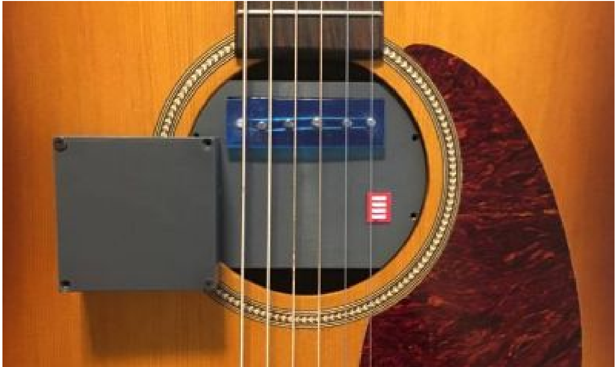
Figure 2 The enclosure is shown inserted into the soundhole of an acoustic guitar. The battery pack is shown on the left and the pickup (top) and effects switch (right) can also be seen.
