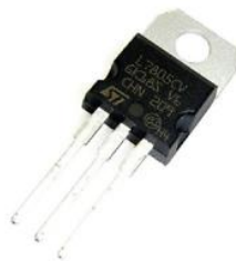
Figure 3: Physical view of MC7805 Voltage Regulator
