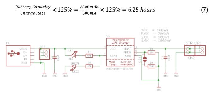
Figure 7. Battery Charger Schematic[12]
