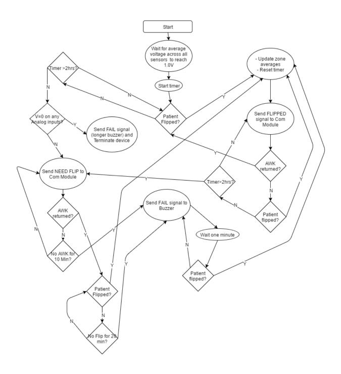
Figure 8. Flow chart of Microcontroller software
