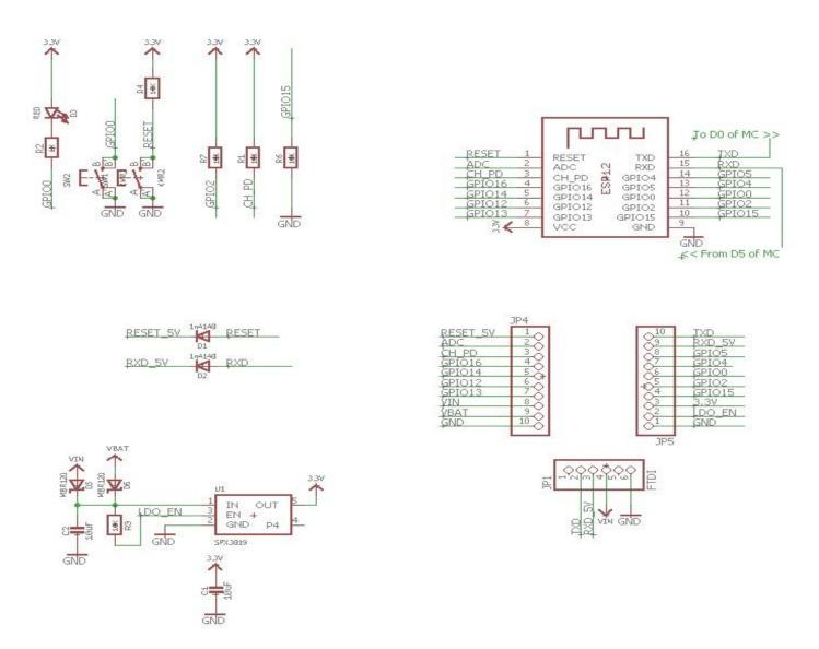
Fig. 10 Schematic of Adafruit ESP8266 breakout[7]
