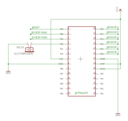
Figure 9. Microcontroller Schematic
