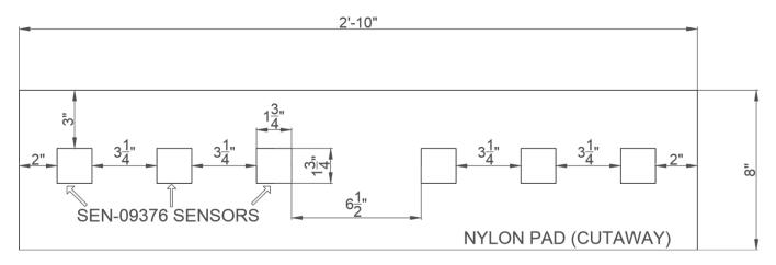
Figure 3. Mechanical Placement of Force Sensors
