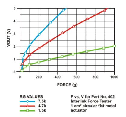
Figure 6. Voltage vs. Force for Different Resistor Values of SEN-09376
