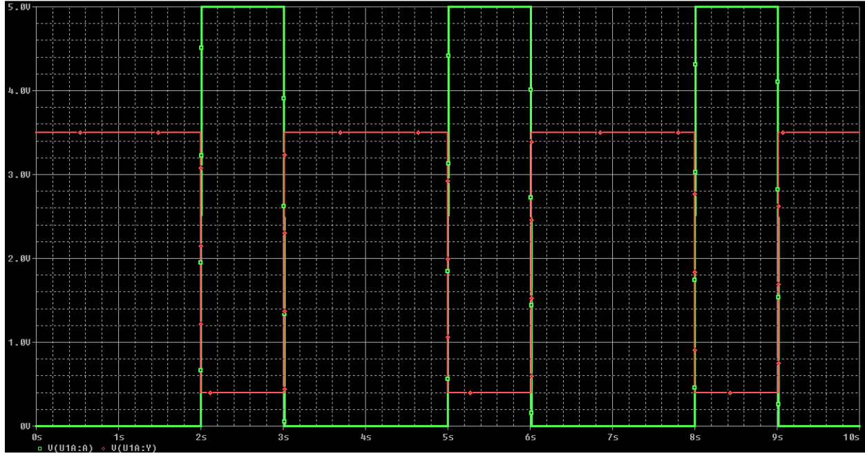
Figure 19. Simulation Result of Inverter Input Voltage (Green line) and Output Voltage (Red line)
