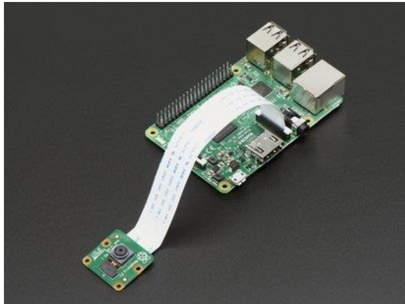
Figure 3. Raspberry Pi Camera module V2 connection with Raspberry Pi[10]
