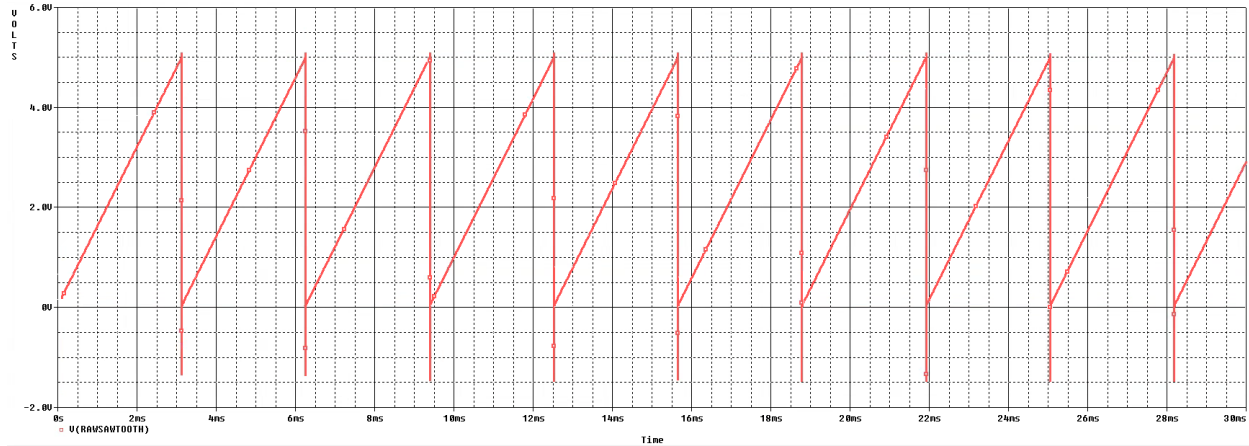
Figure 8: OrCad Simulation of Voltage Controlled Oscillator Sawtooth Wave from 0 to 5 V
