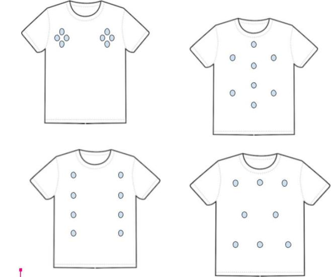
The top left figuration is the easiest design since the microphones are close together and are probably the most comfy since they don't cause the shirt to be constricted as much but spatial resolution is lost they are close together. The bottom right will have the most spatial resolution but will be the hardest to design since the microphones need to be transmitting data and if there are wires connected all over the place, it will make the shirt more constricting in movement.
