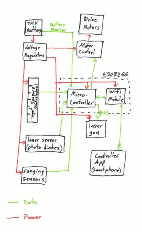
Figure 1: Block Diagram
