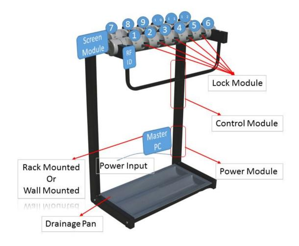
The draft above shows a rough schematic of the system, with the physical rack and various modules inside. The rack/system will be approximately 1.2m wide and 0.7m deep, height will be determined by the type of umbrella used but estimated around 1m tall.
