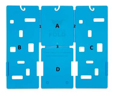
We plan to install our control circuits, power circuits, and all wires below board A(since board A is the only board that stays still during folding process). Three servo motors at edge 1,2 and 3 to flip board B, C and D. Four IR sensors will be mounted on top of board A, B, C and D to detect presence of clothes. Additional two IR sensors will be mounted on the left edge of board B to detect motion of human arms and hands.
